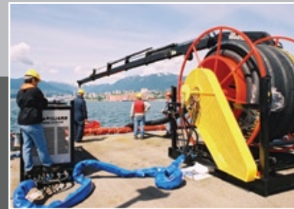
▲ Floating Hose Reel deploying an RBS TRITON™ 50 Skimmer Head
